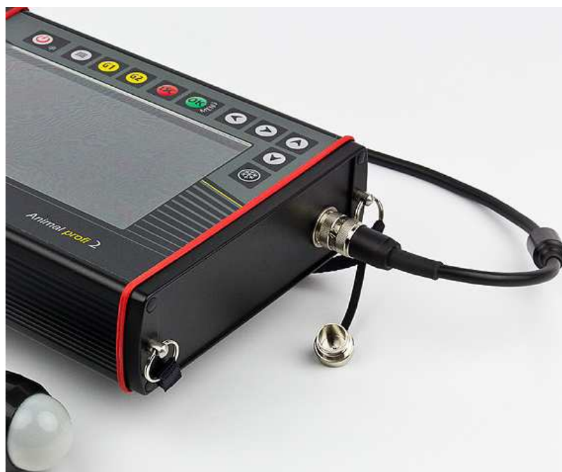
View of the head connector correctly screwed
